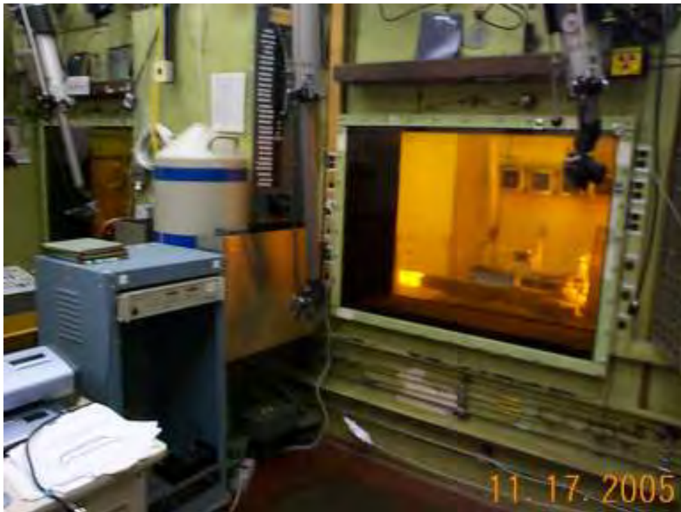
Figure 2. Exterior View of AGHCF Hot Cell
